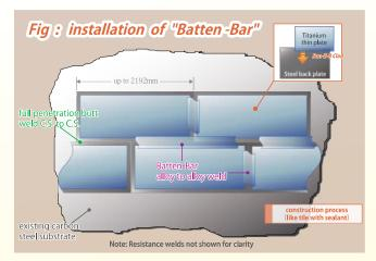
"Batten Bar" design is new construction for FGD. Fabricated plate sizes range from 48" to 144" wide x (up to) 480" long. It can be fabricated in flat or rolled plates and can be sheared or bent to fit any particular design application. Typically, resistance welds are spaced at 6" on centers across the width of the plate for the entire length of the plate to clad the alloy sheet to the full carbon steel backer
