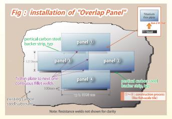
In retro-fit construction for FGD, Resista-Clad Plate is fabricated in what is called an "Overlap" design. Fabricated sheet sizes range from 48" wide x (up to) 240" long. It can be fabricated in flat sheets or rolled sheets and can be sheared or bent to fit any particular design application. Typically, two (2) resistance welds would be made on one long side of the alloy sheet to clad the alloy sheet to the 4" wide partial carbon steel backer plate.
